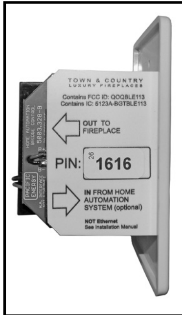
Figure 20: Wall switch with PIN number.
