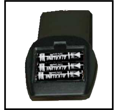
Figure 6: Proflame 2 remote control battery bay.
