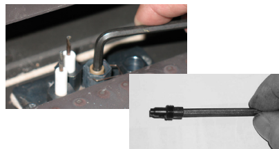
Diagram 2: Slide burner assembly to the right—then remove.
