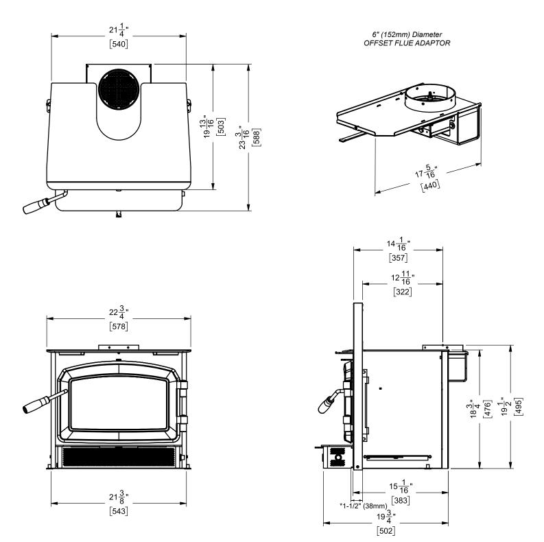
\*Measurement from back of faceplate to fuel door opening
